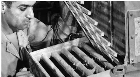
This Drawer-type Grate Magnet is installed in the feed duct and hood of a micro-atomizer.
